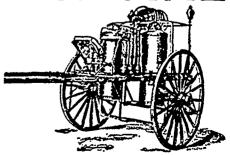
This machine is the most owerful fire fighter. It has two cylinders, 40 gallons capacity each. The combination of chemicals will not freeze, renders material with which it comes in contact non-inflammable, and will not corrode when not in use. For full particulars, write to the Head Office of the Company at Kingston.
