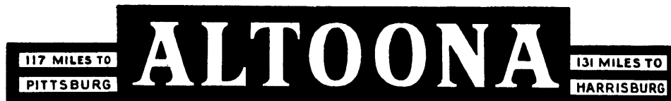
Style no. 3, as used on the Pennsylvania Railroad. White letters on black ground. This sign is 12 ins. high by 6 ft. long. Length varies with number of letters in name of station.
