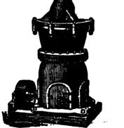
Central Shaft with Crusher-Head supported from top instead of at lower end.
