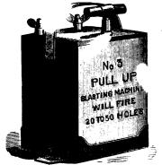
Electric Blasting Apparatus.
