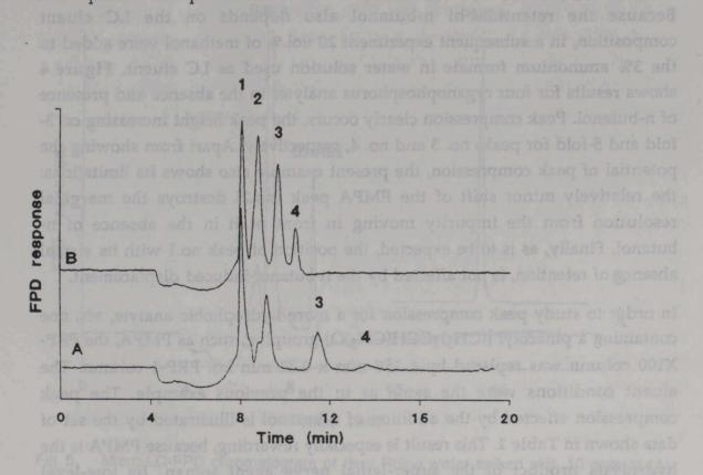
Fig. 4. Micro-LC-FPD chromatogram of several organophosphorus acids. A, without and B, with 9% n-butanol in sample; Column, 300 mm x 0.32 mm i.d. PRP-X100; eluent, 1% formic acid, 2% ammonia and 20% methanol in water; flow rate, 5  $\mu$ l/min. 1, Methylphosphonic acid; 2, ethyl methylphosphonic acid; 3, isopropyl methylphosphonic acid; 4, diethyl phosphoric acid. Concentrations, 1  $\mu$ g/ml.
