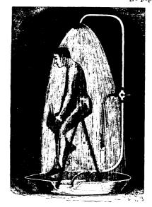
is curved as shown in the engraving and ends in the sprinkler arrangement common to all shower baths. A cock half way up the discharge pipe permits of the water being turned on to the sprinkler or through the hose and nozzle, depending on whether a bath is desired or not.
