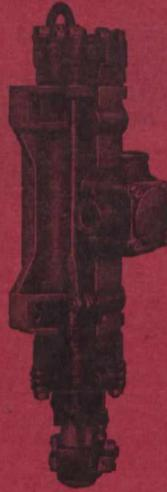
**Materials**—The most carefully selected materials are used in the manufacture of Rand Submarine Drills. Vital cast parts are made of high-grade open-hearth steel castings and steel parts are made of finest selected steels.
