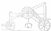
THE NEW STONE AND STUMP EXTRACTOR BREVETED BY LEMIRE.—Capable of litting 18,000 lbs. Has no equal for lifting and carrying stones, etc., for placing stones so as to build ut fence to 5 ft. high and leave the ground in a condition fit for mowing and reaping machines. After the hooks are adjusted on the stones, the only thing to do is to pull it on a stone fence in 10 minutes. The agricultural price moderate. For complete details address:
