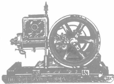
R. & V. Gasoline Engines are equipped with an extra ring over the piston pin. This is one of the desirable features found on all R. & V. "Triumph" Engines. Its value is well understood by all gasoline engine users, as it prevents scoring or ruining of cylinder. This, and other features make the "Triumph" the best gasoline engine for the farm.
