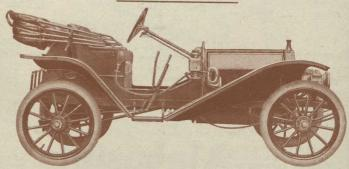
4-Cylinder 20 H.P. Sliding Gears **Bosch Magneto**
