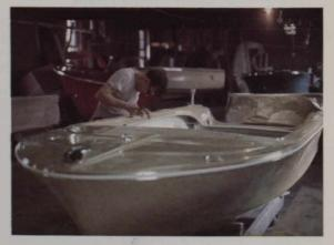
Fibreglass has replaced wood in the building of many boats.
