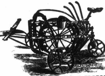
**DITCHING MACHINE, FOR UNDERDRAINING.**
