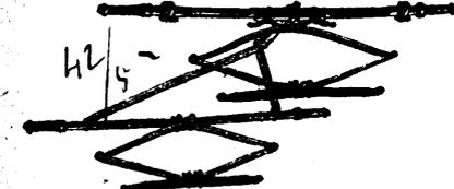
All hung with our Improved Perfect Mangle Plate Springs, setting body two inches lower than formerly, and plates tapered to do away with all quick upward spring or undue motion. The result of our many years' experience practically applied for the benefit of the driving public. A perfect riding buggy, neat and stylish in appearance. Light and strong in use. For sale by all the leading carriage makers.
