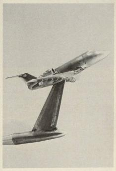
Tests on scale models of the Challenger were done at NRC's wind tunnels operated by the National Aeronautical Establishment. Altogether, it took 1,800 hours of wind tunnel time to arrive at the final configuration, a design close to aerodynamic perfection.
