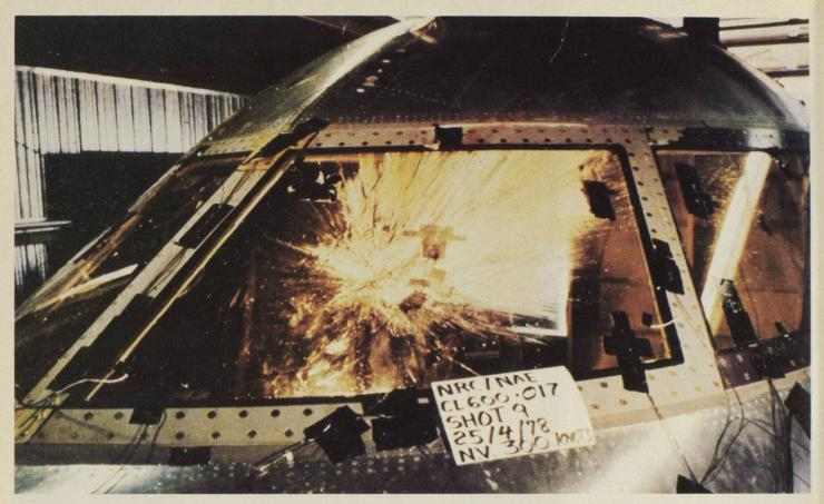
One of the services provided by NRC's National Aeronautical Establishment provides valuable information on whether aircraft structures will stand up to impact with birds, a common hazard of the airways. A large pneumatic cannon fires chicken carcasses at speeds up to 990 km/h. On the basis of the information gained from these tests, Canadair can now be certain that its Challenger will safely withstand bird strikes. (Photo: Canadair Ltd.)
