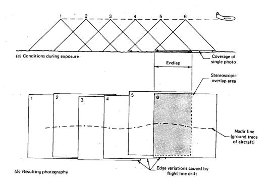
Figure 2. Acquisition of overlapping photographic coverage along a flight strip to provide stereoscopic coverage. (Source: Lillesand, Thomas M. and Ralph W. Kiefer. Remote Sensing and Image Interpretation. John Wiley & Sons. New York. p. 78.)
