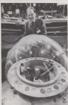
Toronto insurance broker John Ingle shows off a scale model of his invention, a 14-person lifeboat called a Sea Orb, at the Canadian Spring Boat Show held recently in Toronto. Ingle's creation is a circular platform suspended inside a plastic ball about three metres in diameter. It contains provisions for 14 people for six days, self-powered beacons, homing devices, a radio and an airexchange system. It has a toilet and can navigate at up to ten knots an hour.
