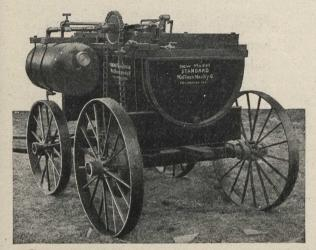
"New Model Standard." A general orchard and vineyard machine which possesses sufficient power and capacity for all ordinary apple trees.
