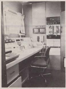
To ensure a reliable flow of information to and from the site of a major derailment, CN Rail has developed the experimental communications trailer containing radio, telephone, telex and video systems.
