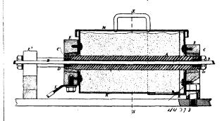
tion in an electrical heater for rods, bars or wires, &c., of an in-sulated refractory tube A, fixed sleeve C, and movable sleeve C<sup>1</sup>, refractory pieces D D<sup>1</sup>, spring G, box made in two parts K K<sup>1</sup>, filled with refractory material, and conductors L L<sup>1</sup>, the whole substantially as and for the purposes set forth.
