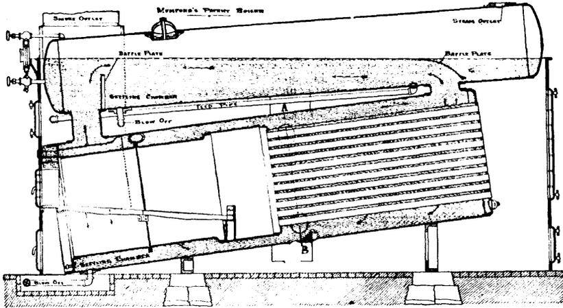
Usually built with a sheet-steel case, but if prepared the case may be left off and brick-setting substituted.
