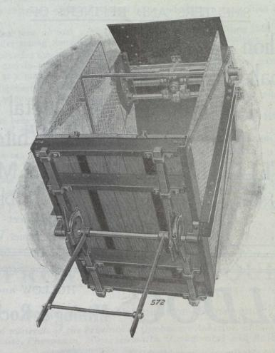
Made to pass provincial government inspection, and in various styles to suit your conditions, with or without rails, and with wire screen or steel plate sides and single or double sets of doors.
