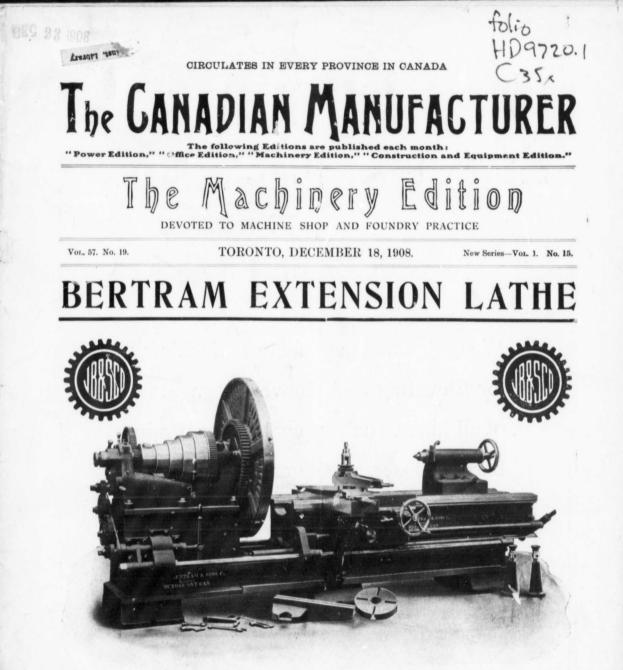
The gap may be narrowed or widened to suit the demands of the work. With the bed extended the machine will swing 55 inches and admit 11 feet clear of face-plate. With the sliding bed moved close to the faceplate the lathe will swing 28 inches over the shears and will handle such work as could an engine lathe of that size. It operates easily and has every wanted lathe convenience. Write for descriptive circular.
