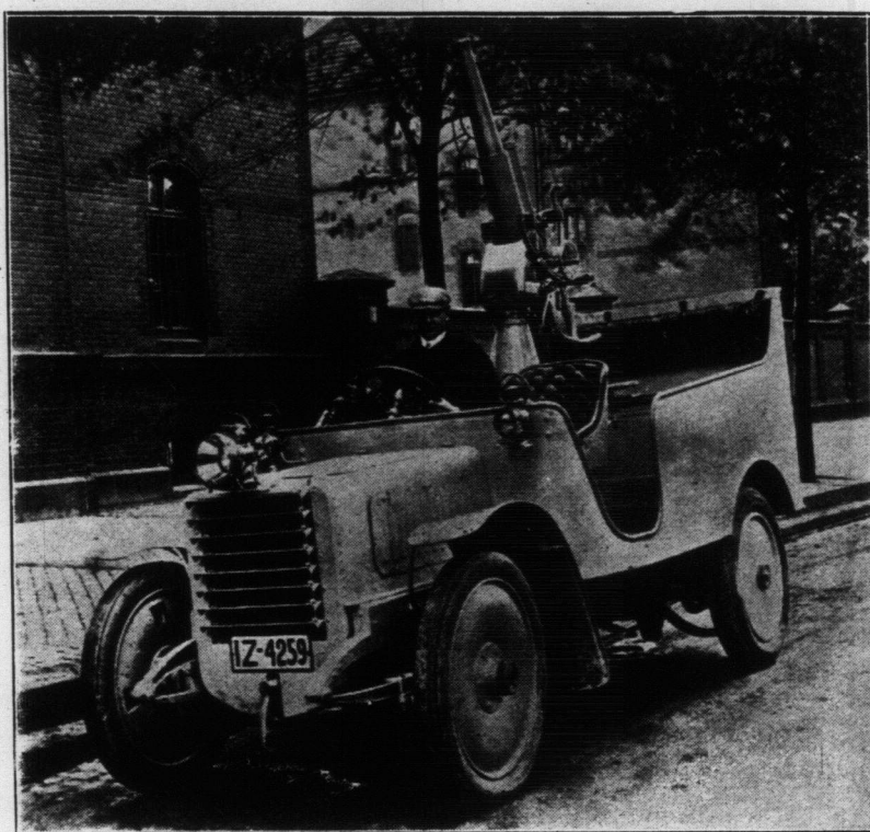
PHOTO OF A QUICK-FIRING GUN MOUNTED ON A MOTOR CAR USED BY THE GERMAN ARMY FOR FIRING AT AIRCRAFT.
