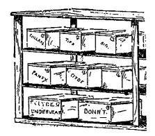
The counter shown in the engraving gives a very clear conception of the manner of its construction. A long table on "legs" might explain it, the top being a board or boards, thick enough and kiln-dried to prevent warping. The supporting pieces need not be wider than three inches. three inches, and about three-quarters of an inch thick. The same material may be used for shelving, this being covered with screen
