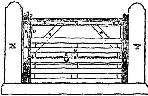
THE above is an engraving of a self-regulating gate designed especially as a convenient and safe arrangement for the season of deep snow, when ordinary gates get blocked up, and are very troublesome. It was invented and patented by E. & S. Stovel of Mount Forest, County of Grey, from whom the right of manufacture and use can be obtained, on terms set forth in their advertisement, which appears on the last page of our present issue.
