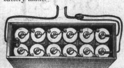
This cut illustrates the most practical method of using HI-PO Waterproof Dry Batteries, namely, in double series, thus, by means
