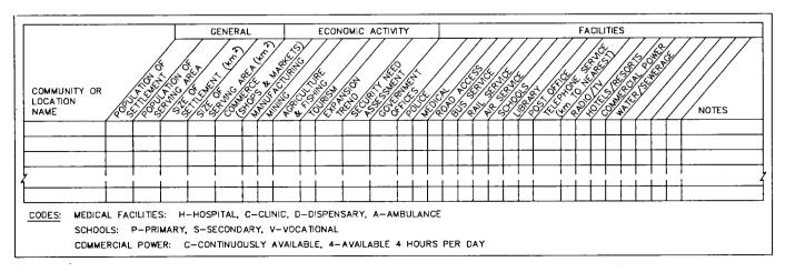
FIG 4-2 Typical Worksheet to Inventory Potential Locations for New or Expanded Telephone Service
