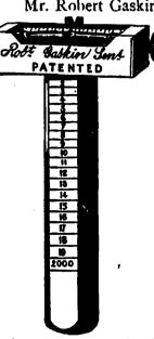
Mr. Robert Gaskin, sr., of St. John N. B., has just patented a simple combined wind gauge, plumb and elevation back sight for fire-arms and ordnance, in which our readers will doubtless be interested. The ordnance appliance shown on the left, will, it is claimed, enable the marksman quickly to find the vertical line through the centre of plane of the bore of the gun. By simply traversing the
