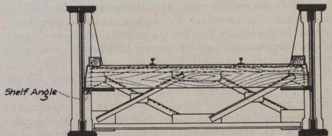
Fig. 2.—Half Deck Plate Girder.
