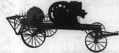
There are many places where there is hoisting to do with a direct line using a rope or cable when a simple and efficient hoist will save a great deal of time, labor and expense. The No. 3 Ideal Hoist will handle loads up to 1500 pounds, and is used with the greatest success for operating single platform elevators, derricks, ice,
