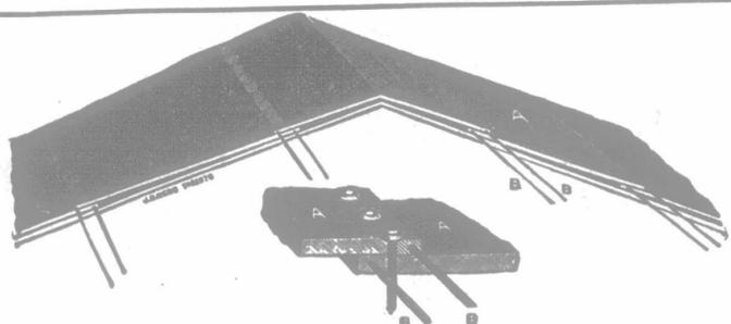
A shows method of laying Red Star Brand Wire-edged Ready Roofing, with 2-inch laps secured by nailing two inches apart. B B shows the joints or laps—a very desirable feature, especially in localities where high winds prevail.
