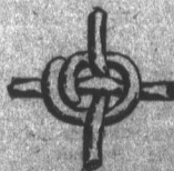
This cut shows the knot or lock in the Page "Empire" Fence.
