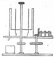
The cylinder through the bottom must be large enough to allow the small wheel by which the machine is driven to pass freely through it, and the tub must be of sufficient diameter to allow of the basket and spindle of the turbine to be freely lifted in and out of it, so that when a charge is done, the basket and spindle may be lifted out, and the sugar emptied out of it, and be replaced ready for another charge, without jamming in the cylinder and against the sides of the tub.
