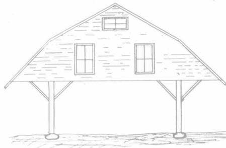
FIGS. IV AND V—A SHED BUILT "UMBRELLA STYLE" PROVIDING TOOL-ROOM ABOVE
