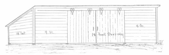
FIG. VI-THIS SHED IS BUILT OF ROUGH LUMBER, NAILED ON POSTS, AND CAN BE PUT UP AT VERY SMALL COST
