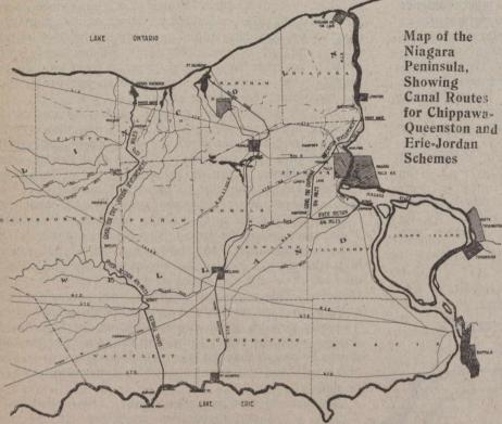
to adopt for the Hydro Power Canal, the route shown on the accompanying map. This route is about 1234 miles long, with the intake on the Niagara River at Hog Island, Chippawa, about two miles above Niagara Falls, and the tailrace on the Niagara River about one mile above Queenston. The intake will be in what is known as the Grass Island pool of the Niagara River. The mean monthly elevation of this pool varies about 1 ft.
