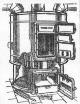
The walls of the fire-pot are straight and ashes do not bank against them to stop the radiation of heat from the burning coal. The doors of
