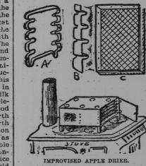
two inches broad, bent in the form illustrated, and riveted in box inside, one at each end and one in middle. The end supporters of sieves are bent as in the cut, to extend down and serve as feet for the drier. The middle supporter need not reach below box.
