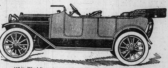
116-in. Wheel Base-34 x 4-in. Tires-Silent Chain Driven Motor Gears Cork Insert Clutch-4 x 5-in. Motor.
