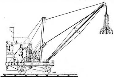
"Lancaster" hand power placer apparatus and above is illustrated a steam power placer digging machine which more rapidly furnishes the gold bearing gravel to the sluicing apparatus. This latter is built in sizes to correspond with the capacity of the automatic digger; power for same is transmitted to the sluicing apparatus thus saying manual labor.
