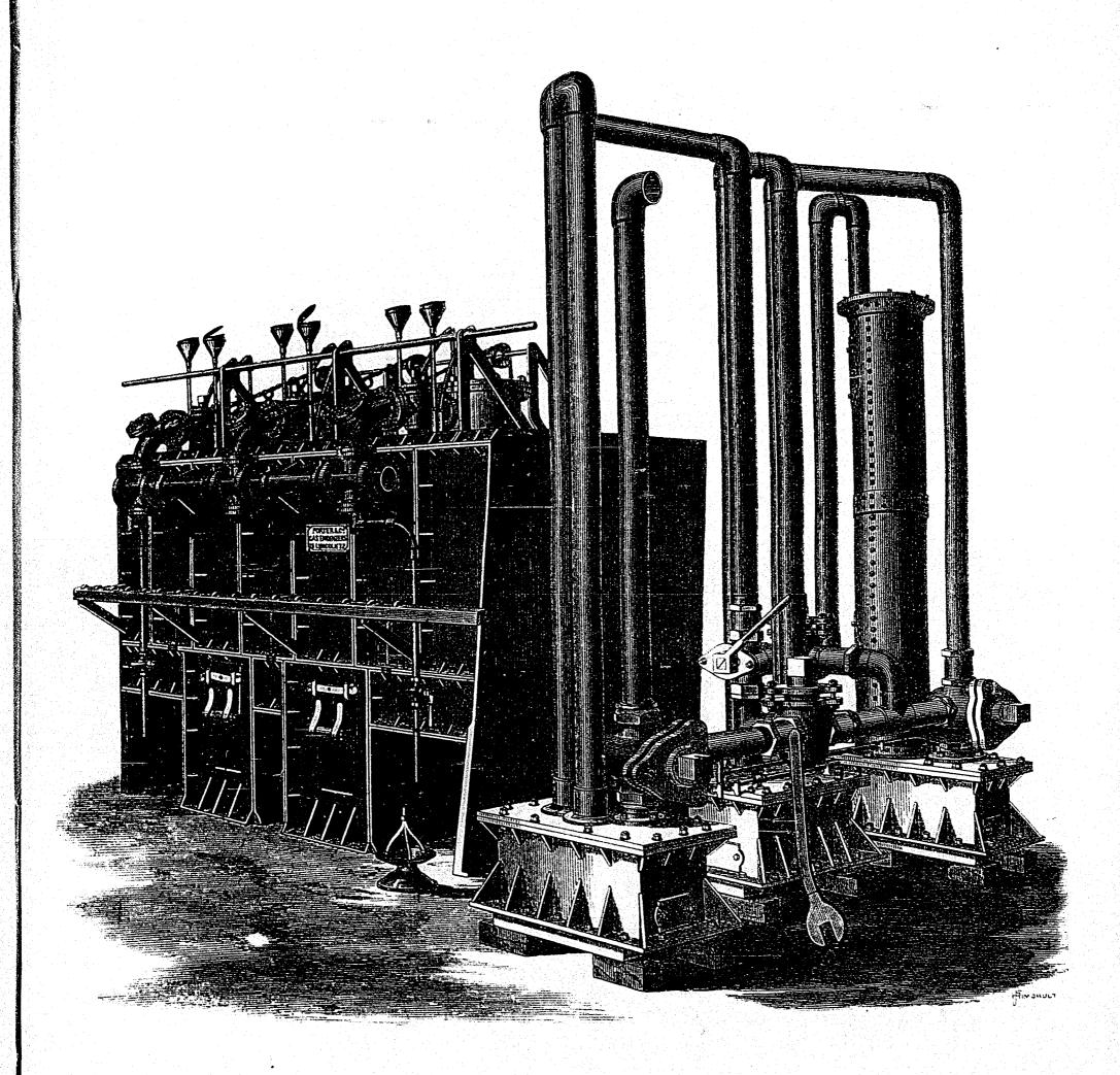
APPARATUS FOR MANUFACTURING GAS ON SHIPBOARD.
