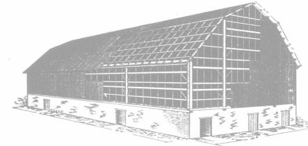
This cut shows an up-to-date Barn Construction, 40 feet by 70 feet, and the method of covering with Corrugated Sheets. The framework is light, as the corrugated sheets, when nailed in place, made the building very rigid. This drawing is made from actual plans and the barn has been built many times with splendid results.
