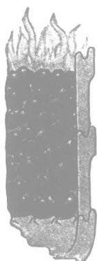
Straight Walls Fire-pot of "SUNSHINE"
