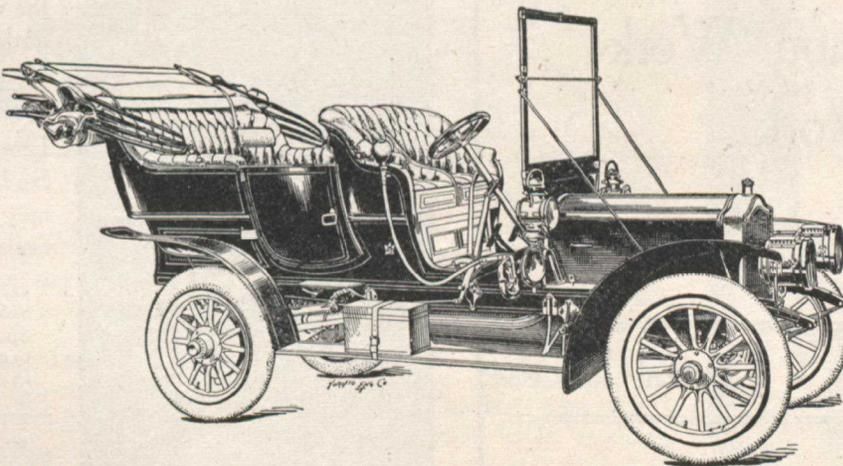
In each of the metal-to-metal disc clutch, shaft drive, selective sliding gear transmission, nickel steel in all gears and shafts, powerful double brakes on rear wheels, positive lubricating and water circulating systems.
