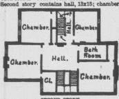
SECOND STORY. (with fireplace), 14x15; chamber, 14x14; chamber, 10x14; chamber, 13x15; closet off each chamber; bathroom, Estimated cost of building, \$8,000.
