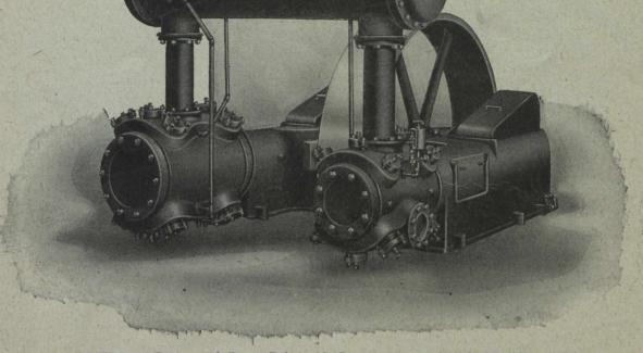
Class "PLB-2" Cross Compound, Power Driven Air Compressor, equipped with "Circo" Silent Leaf Inlet and Outlet Valves, Enclosed Dust-proof Frames and Splash and Flood Lubrication System.
