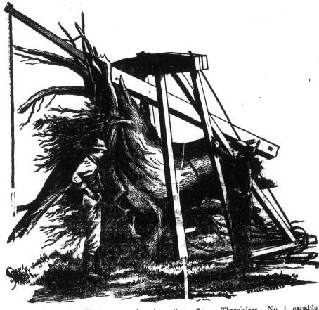
Will take out 20 to 50 stumps per day, depending on size. Three sizes. No. 1, capable of drawing any stump, \$120. No. 2, for stumps 2 feet 6 inches, \$90. No. 3, for 18 inch stumps, \$70. The largest sizes will take out the smallest stumps, but they are constructed much stronger and heavier.—Apply to PLUMMER & PACEY, Waggon Makers, London, or to W. WELD, Agricultural Emporture. Agricultural Emporium.
