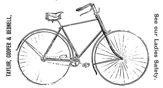
THE POPULAR RAGLAN SAFETY, built especially for Canadian Trade. The finest Wheel for the price, and guaranteed for a year. Frame of Weldless Steel Tubing and Steel Stampings, Ball Bearings throughout, Ball Socket Head, Cushion Tire, Garford Saddle. Price, \$85.00. Special.
