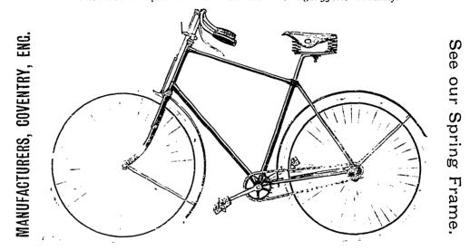
RAGLAN LEADER SAFETY—Cushion and Pneumatic Tires, 30 inch Front and 28 inch Rear Wheels, Extended Wheel Base, Ball Bearings throughout, built for Canadian Roads and general road use, being very light. Warranted. Price, Cushion Tire, \$140.00. Pneumatic, \$160.00, including Garford Saddle Dunlop, Heale's or McIntosh Pneumatic Tires.
