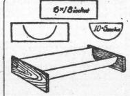
inches in diameter. Nail these pieces together, using the semicircles for the form of the trough. The sheet iron is then bent into these forms to make the body of the trough. A 1 by 2 inch strip nailed between the ends close to the outside edge of the iron, to which it may be tacked, adds greatly to the strength of the trough. The above makes a very convenient, light and economical trough for farrowing time and has given the writer very satisfactory results .- Farmer.
