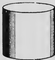
FIG. 5.—Kilogram, made of an alloy of platinum and iridium. Height and diameter each 1.5 inches.
